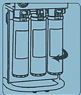
Twist clockwise for removing old cartridge
