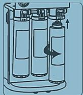
Twist anti-clockwise to fit in new cartridge
