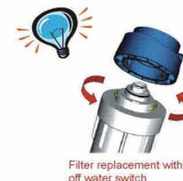
Filter replacement without shutting off water switch
